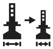
The compact design of the Ultinon Essential LED bulbs make installation simple. Even in the smallest headlamps, you'll have space to fit these bulbs. Because of the flexible copper braids of the heat sink, and the curved control box, you can fit your new LED lights in cars where other products would be too bulky.
