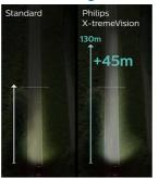
With its optimized high-precision fillament geometry, up to 13 bar high pressure gas filling, high precision coating and high quality UV-Quarz glass, Philips X-tremeVision headlights set a new milestone in automotive lighting. They are engineered for the ultimate performance and uncompromising visibility.
