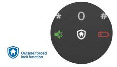
Before leaving home, you can touch the outside forced lock button to enable the function. In this mode, opening the door from inside will trigger an alert. This feature can effectively remind you of security risks and upgrade the level of home security.
