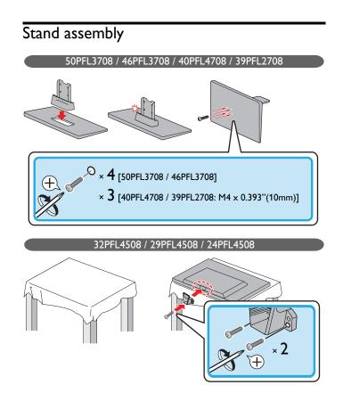
Attaching the base You must attach the base to the unit to have it as a table top unit. Be sure the front and rear of the base match the proper direction. For large screen TVs, at least 2 people are required for these steps.
