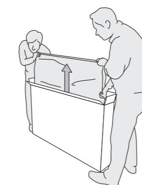
Prepare a table and cover the top of it with a table cloth, blanket or such to avoid damage to the TV set. Support both sides of the TV set and, move it onto the table.
