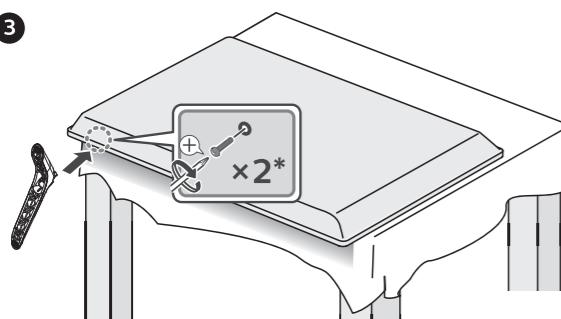
**!** Fasten the stand to the TV with 2 screws (included). While fastening the screws, hold the stand to prevent it from falling.
