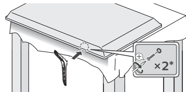
**!** Fasten the stand to the TV with 2 screws (included). While fastening the screws, hold the stand to prevent it from falling.
