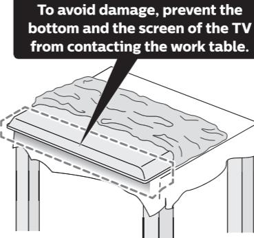
**To avoid damage, prevent the bottom and the screen of the TV from contacting the work table.**
