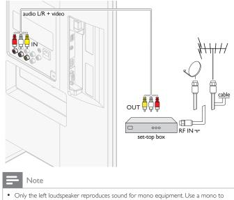
stereo adapter (not supplied) for sound reproduction via all internal loudspeakers.When you connect cables, match the cable colors to the connectors on the TV.
