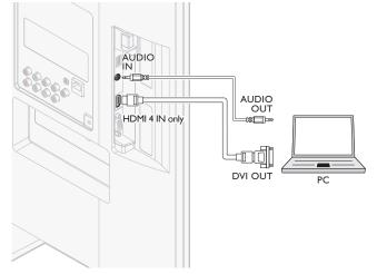
If you connect a PC with an HDMI or Display Port (HDMI-Display Port conversion cable) connector.
