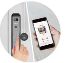
The"#" key is used both as a doorbell button and a "#" key. When the door lock is in sleep mode and pressing the "#" key can activate the doorbell, and the camera will immediately capture the photo and uploads it to the Smart Life App. After viewing the logs and confirming the visitor's information, you can unlock the door remotely through the App with a singel tap, allowing the visitors to enter the door easily.
