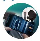
Philips Alpha-VP-5HWS equips with a wideangle camera and two low-power infrared fill lights. It has daytime mode and night vision mode. When the light is dim, the infrared fill light will automatically turn on, switch to night vision mode, and recognize the facial features within 1 meter from the lock end.
