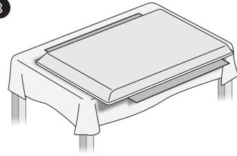
**!** Carefully lay the TV set, with the screen side down, on the front cardboard as shown in the figure.
