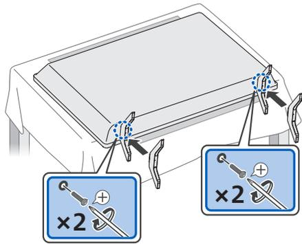
**!** Fasten the stands to the TV with 4 screws (included). While fastening the screws, hold the stand to prevent it from falling. Both stands now be securely fastened.
