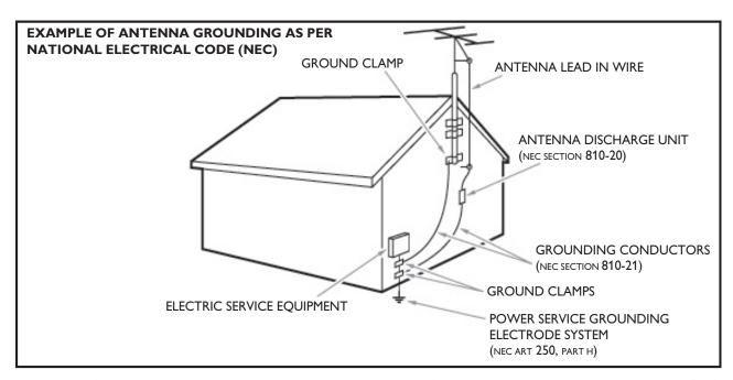
**Note to the CATV system installer:** this reminder is provided to call the CATV system installer's attention to Article 820-40 of the NEC that provides guidelines for proper grounding and, in particular, specifies that the cable ground shall be connected to the grounding system of the building, as close to the point of cable entry as practical.
