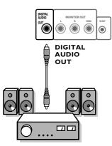
Connect a Digital MultiChannel Surround receiver to the **DIGITAL AUDIO OUT** connector at the bottom of the TV.
