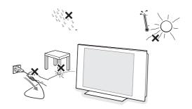
Do not insert the power plug in a wall socket or hang the TV to the wall before all connections are made.
