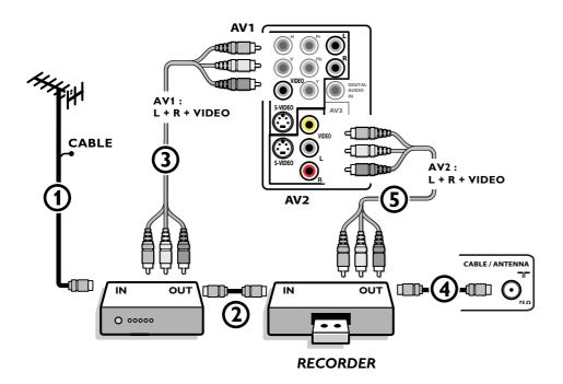
Connect the RF antenna cable (1) of the RF IN socket of your other AV device.
