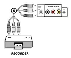
The **MONITOR OUT** connector can be used for a daisy chaining or to record programs from your TV **(3)**. Only when a recorder is connected to **MONITOR OUT** it is possible to record an analog program from your TV. See Record with your recorder, p. 37.
