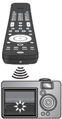
1. Point the IR transmitter of the remote control towards the lens of the digital camera (or cell phone camera).
