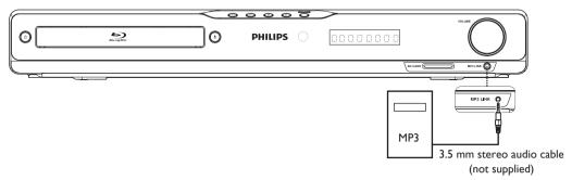
Connect a 3.5mm stereo audio cable (not supplied) to the MP3 LINK jack on this unit and the headphone jack on your portable media player.
