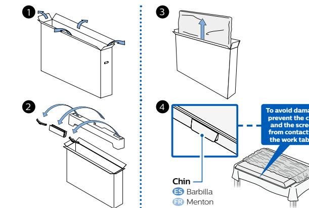
Cover a table top with a cloth or blanket to avoid damage to the TV screen. Hold both sides of the TV set to place on the table.
