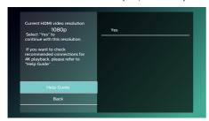
Playback is possible on conventional 2K High-Definition TV's, however, the picture quality will be down-converted to match the TV resolution (720p / 1080i / 1080p).
