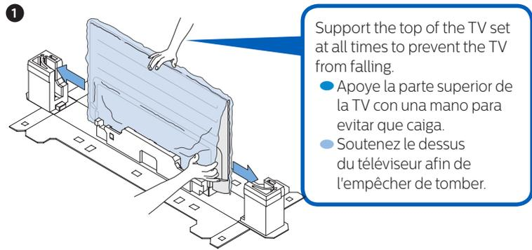
Support the top of the TV set at all times to prevent the TV from falling.
