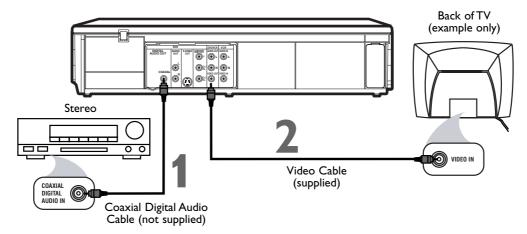
Connect a coaxial digital audio cable (not supplied) to the DVD/VCR's COAXIAL DIGITAL AUDIO OUT jack and to the COAXIAL DIGITAL AUDIO IN jack on the Stereo.
