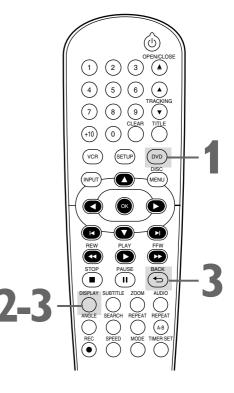
Press DISPLAY repeatedly or press BACK to to remove the display.
