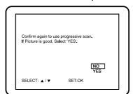
Confirm your setting, then press OK. The menu will disappear and the Progressive Scan function will be activated. If you do not press any buttons for 15 seconds, Progressive Scan will switch to OFF.
