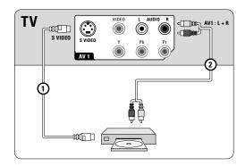
• When using the **S-VIDEO** connector, **do not** connect any device to the **AV VIDEO** input that you are usting.
