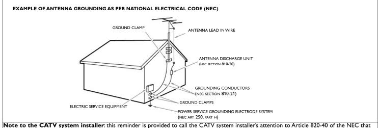
Note to the CATV system installer: this reminder is provided to call the CATV system installer's attention to Article 820-40 of the NEC that provides guidelines for proper grounding and, in particular, specifies that the cable ground shall be connected to the grounding system of the building, as close to the point of cable entry as practical.
