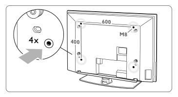
2 Should the plastic discs obstruct the VESA bracket, you can unscrew these 4 discs.
