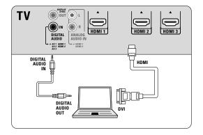
11.13.4 Equipped with a HDMI connector
