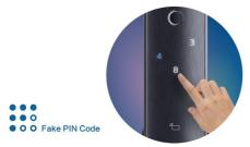
Philips EasyKey comes with the feature of Fake PIN Code technology which allows you to enter random number combinations to successfully get identified as long as there is consecutive input of the real password. This feature can effectively prevent peeping and safeguard your real password.
