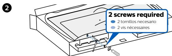
**!** Prior to attaching each stand, make sure to peel off the protective film where each stand goes in so it will not get stuck between the unit and the stand. Fasten the stand to the unit with 2 screws each (included).
