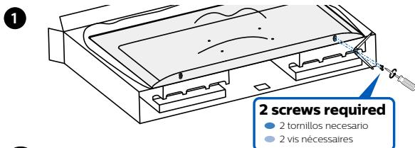
**!** Prior to attaching each stand, make sure to peel off the protective film where each stand goes in so it will not get stuck between the unit and the stand. Fasten the stand to the unit with 2 screws each (included).
