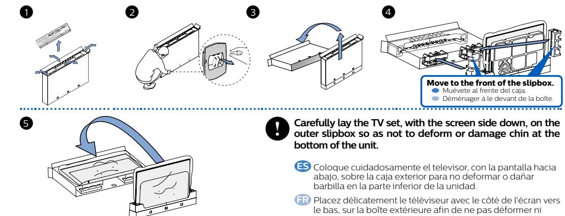
! Carefully lay the TV set, with the screen side down, on the outer slipbox so as not to deform or damage chin at the bottom of the unit.
