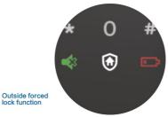
Before leaving home, you can touch the outside forced lock button to enable the function. In this mode, opening the door from inside will trigger an alert. This feature can effectively remind you of security risks and upgrade the level of home security.
