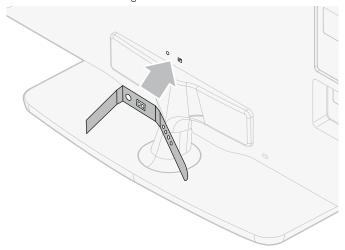
2 Pass cables through the cable management tie to avoid tangles.
