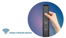
With a touch sensor and an infrared sensor on the handle, the door could be opened much easier. Once the hand touches the touch sensor and the infrared sensor detects the obstruction, the lock will open.
