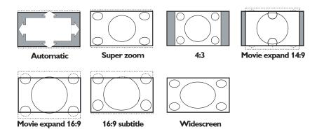
Super Zoom, Movie expand 14:9, Movie expand 16:9 and 16:9 Subtitle makes the picture fill the screen as much as possible. It is recommended to press the cursor up/down key to adjust the picture position on the screen.
