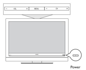
Should your remote be lost or broken you can still change some of the basic settings with the buttons on the top of your TV. Press the power switch  $\phi$  to switch the TV on.
