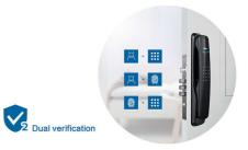
In the dual verification mode, you could open the door with any two verification methods (facial recognition, fingerprint, and PIN code), which provides double protection for home security.
