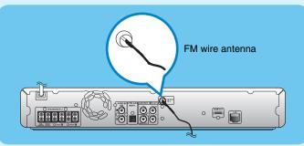
Connect the supplied FM wire antenna to the inner pin of the FM ANT 75  $\Omega$  jack. Extend the wire for optimum reception.
