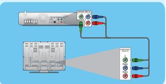
\*1) This unit is compatible with the progressive scan system. The feature provides you with the higher quality pictures than traditional output system does. To utilize this feature, a component or an HDMI connection is required. Refer to the "Video Resolution" on page 41 in the user manual to set the resolution.
