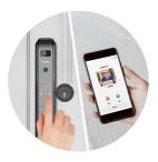
The"#" key is used both as a doorbell button and a "#" key. When the door lock is in sleep mode and pressing the "#" key can activate the doorbell, and the camera will immediately capture the photo and uploads it to the Smart Life App. After viewing the logs and confirming the visitor's information, you can unlock the door remotely through the App with a singel tap, allowing the visitors to enter the door easily.
