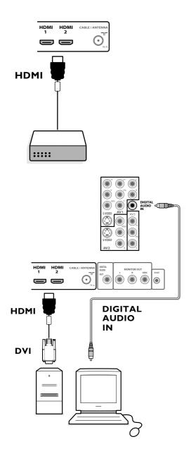
HDMI is the leading new standard for Digital video and audio interconnection. To the **HDMI** connector you can connect HDMI devices such as a Set Top Box or compatible DVD-R or DVD player with HDMI, or DVI-equipped devices like a computer.
