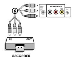
The **MONITOR OUT** connector can be used for a daisy chaining or to record programs from your TV **(**.). Only when a recorder is connected to **MONITOR OUT** it is possible to record an analog program from your TV.
