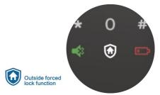
Before leaving home, you can touch the outside forced lock key to enable the function. In this mode, opening the door from inside the room will trigger an alarm. This feature can effectively warn you of security risks and upgrade the level of home security.
