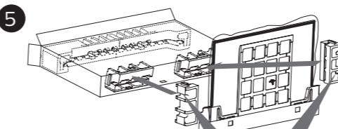
Side cushions, place them inside slipbox ( To give strength to place TV on top of carton box for stands installing ).
