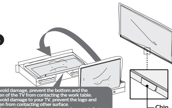
To avoid damage, prevent the bottom and the screen of the TV from contacting the work table.
