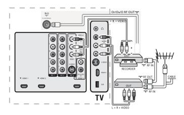
If your recorder has an S-VHS video jack: For improved picture quality, connect an S-Video cable with the S-Video input. Connect the audio cables to the audio L and R input jacks of AV3/side AV.
