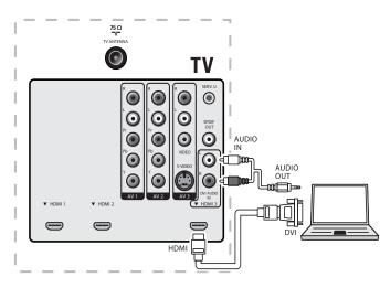
Connect a PC with an HDMI connector
