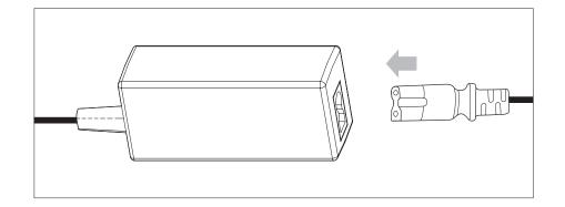
2 Connect one end to the DC IN socket on the main unit.
