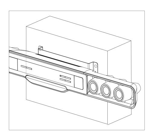
4 Secure the wall mount bracket onto the main unit with 2 supplied screws.
