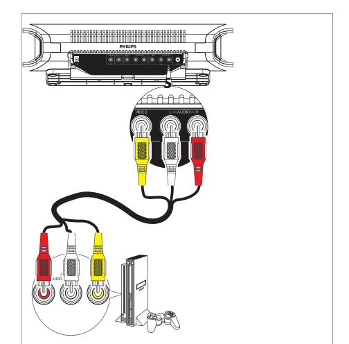
2 Connect the video input socket on the TV to the VIDEO OUT socket with the supplied yellow composite cable.
