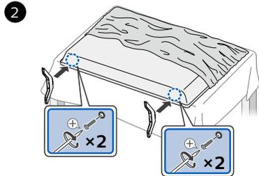
**Fasten the stand to the TV with 4 screws. While fastening the screws, hold the stand to prevent it from falling.**
