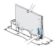
3 Remove the protective film on the bottom of the TV and fasten the matching stand to the TV with 3 screws (included).
