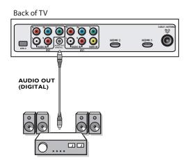
Connect a Digital MultiChannel Surround receiver to the AUDIO OUT (**DIGITAL**) connector at the bottom of the TV.
