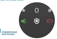
Before leaving home, you can touch the outside forced lock button to enable the function. In this mode, opening the door from inside will trigger an alert. This feature can effectively remind you of security risks and upgrade the level of home security.
