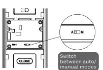
[A] represents Auto mode. The dead bolt will pop up automatically after closing the door and the door will be locked.
