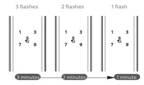
If there are 5 consecutive incorrect inputs of any of the 3 types of verification methods (fingerprint/PIN code/card), the system will be locked for 3 minutes.
