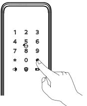
1) Press [#] key before inputting any other numbers. After hearing a voice prompt of "Enter master PIN code", enter your master PIN code and confirm with [#]. Then you are in master mode.
