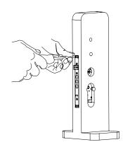
Install the connecting screw tube, and place the square shaft and compressed spring into the hole of the lever. (The square shaft compressed spring must be put towards the lever)
