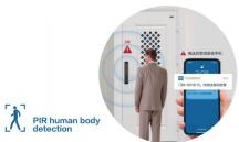
Adopted with the PIR, when someone moves around the front door within 3 meters, the AI humanoid detection algorithm will identify abnormal dynamics by instantly capturing a photo or a video, and simultaneously pushing a message to the APP through the encrypted
