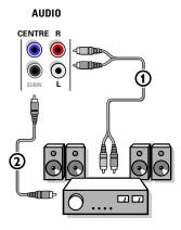
① Connect the audio cable to the multi channel Surround receiver and to AUDIO RECEIVER L and R next to the CENTRE connector of your TV ①.
