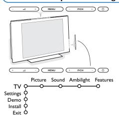
Should your remote be lost or broken you can still change some of the basic settings with the buttons on top or on the right side (according to the type of your set) of your TV.
