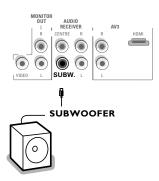
To enhance the sound reproduction of your TV you can connect an externally powered subwoofer (between 20 and 250 Hz).
