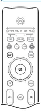
Press the **PIP** button to switch on **Dual screen**, **PIP** or one of the PIP modes according to the format selection made in the PIP format list in the General menu. See Settings, General, p. 8.
