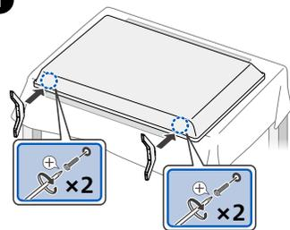
**!** Fasten the stand to the TV with 4 screws (included). While fastening the screws, hold the stand to prevent it from falling.
