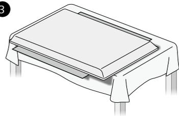
**!** Carefully lay the TV set, with the screen side down, on the front cardboard as shown in the figure.
