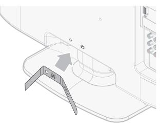
2 Pass cables through the cable holder to avoid tangles.
