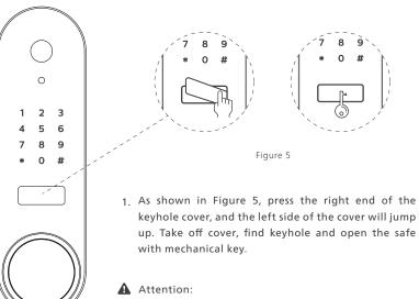
do not place the mechanical key into the safe!
