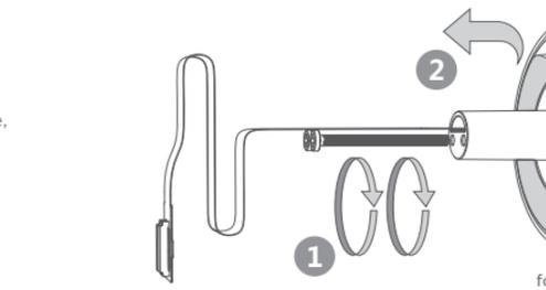
Sort out the connecting cable, then tighten the screw into the sub-unit for 5mm, and tear the foam label protective sheet on the rear side of the sub-unit.
