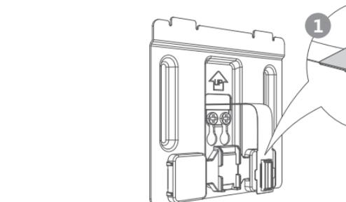
Gently pull out the connecting cable from the inside door, and then peel off the protection film on the back of the sub-unit interface.
