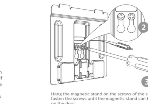
Hang the magnetic stand on the screws of the sub-unit and fasten the screws until the magnetic stand can be fixed firmly on the door.
