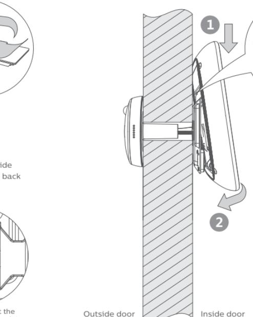
Attention: Align the host device to the magnetic stand from the top to bottom. Tilt the host by 10 degrees and hang it on the steel sheet from top to bottom. The bottom magnet will automatically suck with the host. After installation, gently pull the upper part of the host to check if it is correctly installed.
