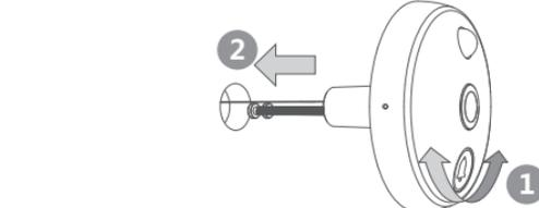
Adjust the direction of the sub-unit from outside and make sure the doorbell button is at the bottom. Then pass the screw and connecting cable through the hole. (If your door is too thick, use a paper tube to pass the cable through the door, then remove the paper tube ). Press hard on the sub-unit to make sure it perfectly adheres to the door, then remove the lens protective film.
