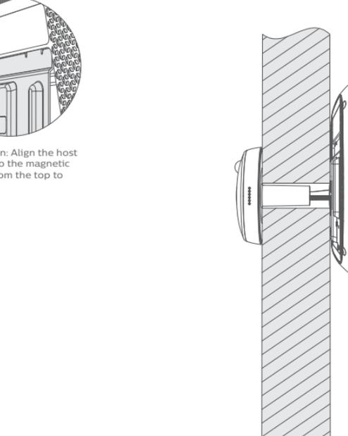
Please hold the bottom of the host with both hands and tilt it upwards by 10 degrees, and then move it against the steel sheet to remove the host.
