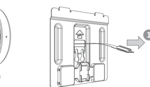
Pass the connecting cable of the sub-unit through the square hole on the magnetic stand from the inside door. ( Do not twist or squeeze the connecting cable.)
