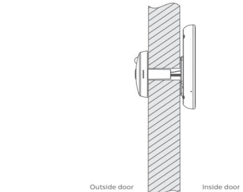
Please choose the proper screw as per the door thickness for sub-unit installation. Short size screw is applicable for a door thickness of 35mm-60mm. Medium size screw is applicable for a door thickness of 60mm-85mm. Long size screw is applicable for a door thickness of 85mm-110mm.
