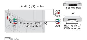
The unit accepts 480i, 480p, 720p, 1080i and 1080p of video signals for this connection.
