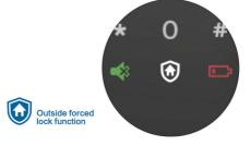
Before leaving home, you can touch the outside forced lock key to enable the function so that opening the door from inside the room will trigger an alarm. This feature can effectively warn you of security risks and upgrade the level of home security.
