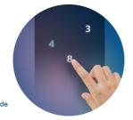
Feature with hidden PIN code technology, Philips smart lock allows you to enter any random number combinations to successfully get identified as long as there is a consecutive input of the real password. This feature can effectively prevent peeping and safeguard your real password.
