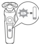
When the battery is almost empty, the battery charge indicator flashes orange and the shaver beeps. At this point there is enough energy left for one shave.
