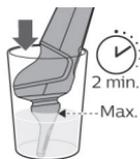
If rinsing the trimming head under the tap is not sufficient, immerse the trimming head in a glass with warm water for a few minutes. Then switch on the appliance and rinse it under the tap.
