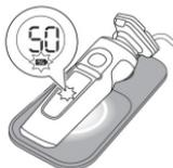
When the shaver is charging, the ring on the pad lights up and the battery charge indicator on the shaver flashes white.
