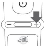
The shaver has a feature that allows you to personalize your settings. Depending on your personal shaving needs, choose between three settings, from low to high: comfort, dynamic or efficiency. When you press the button on the left or right of the display, the segment of the personal comfort settings bar lights up to indicate the selected setting. To select a lower or higher setting, press the button on the left or right of the display.
