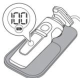
When the battery is fully charged, the battery charge indicator and the ring on the pad light up white continuously.
