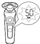
The remaining battery charge is indicated by the battery charge percentage shown on the display.
