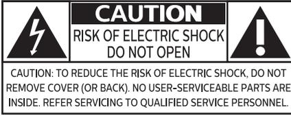
The caution marking is located on the rear or bottom of the cabinet.
