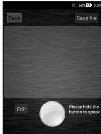
1、 Long press the “Speaker” to talk and release it when talk is over. The audio is automatically converted to text. The audio-to-text conversion interface is shown below:
