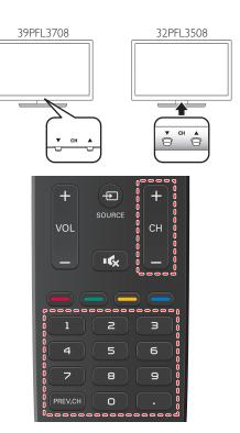
To select Channels by using CH  $\vee/A$  or CH + / -
