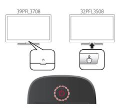
To Turn the TV On from Standby or Off to Standby
